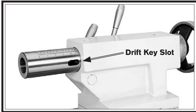
Figure 43. Drift key slot in the side of the quill.
